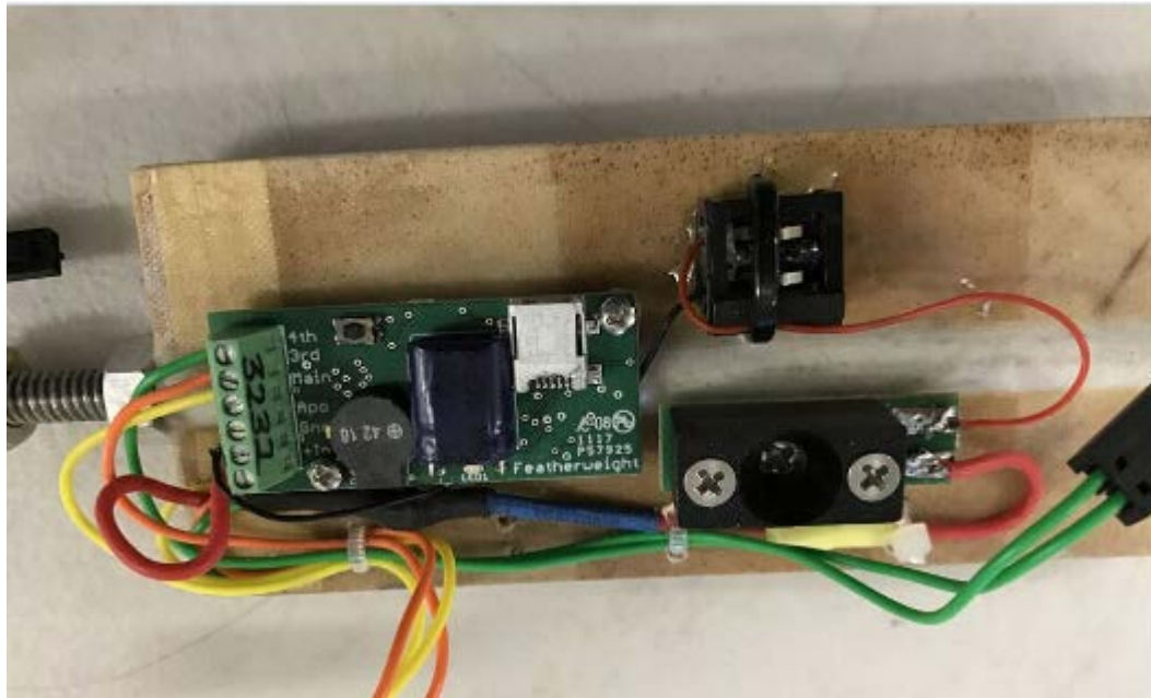
Figure 9 – Raven Altimeter as set up for our subscale flight
