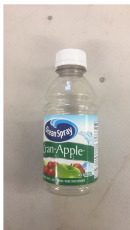
Figure 20 - 10oz Water Vessel, without water: 28 g, with water: 293 g
