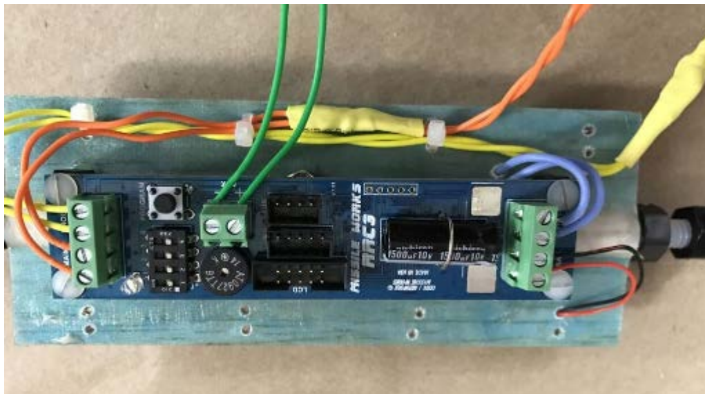
Figure 10 – RRC3 Altimeter as set up for our subscale flight
